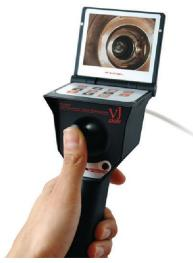
The base imaging unit houses the main PCB, camera articulation controls, video monitor and power supply. *Source: RF System Lab*
