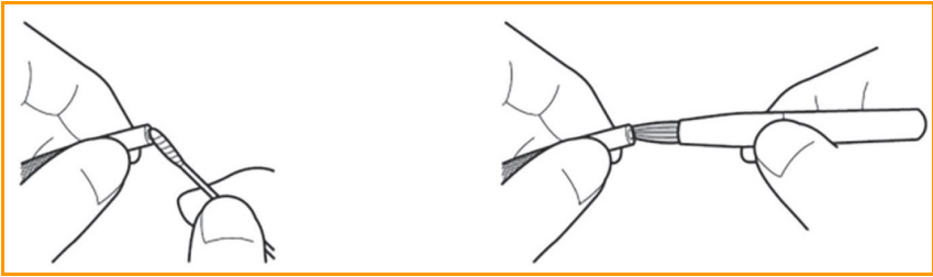
Fig. 8-1 Cleaning the camera at the end of the insertion tube
