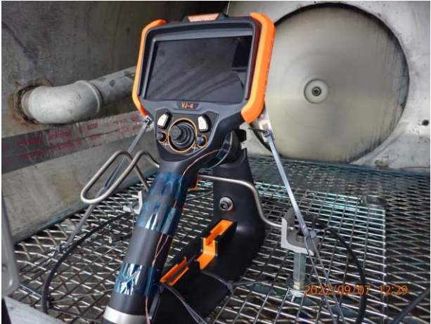
EUT in Test Chamber After Explosive Atmosphere Test
