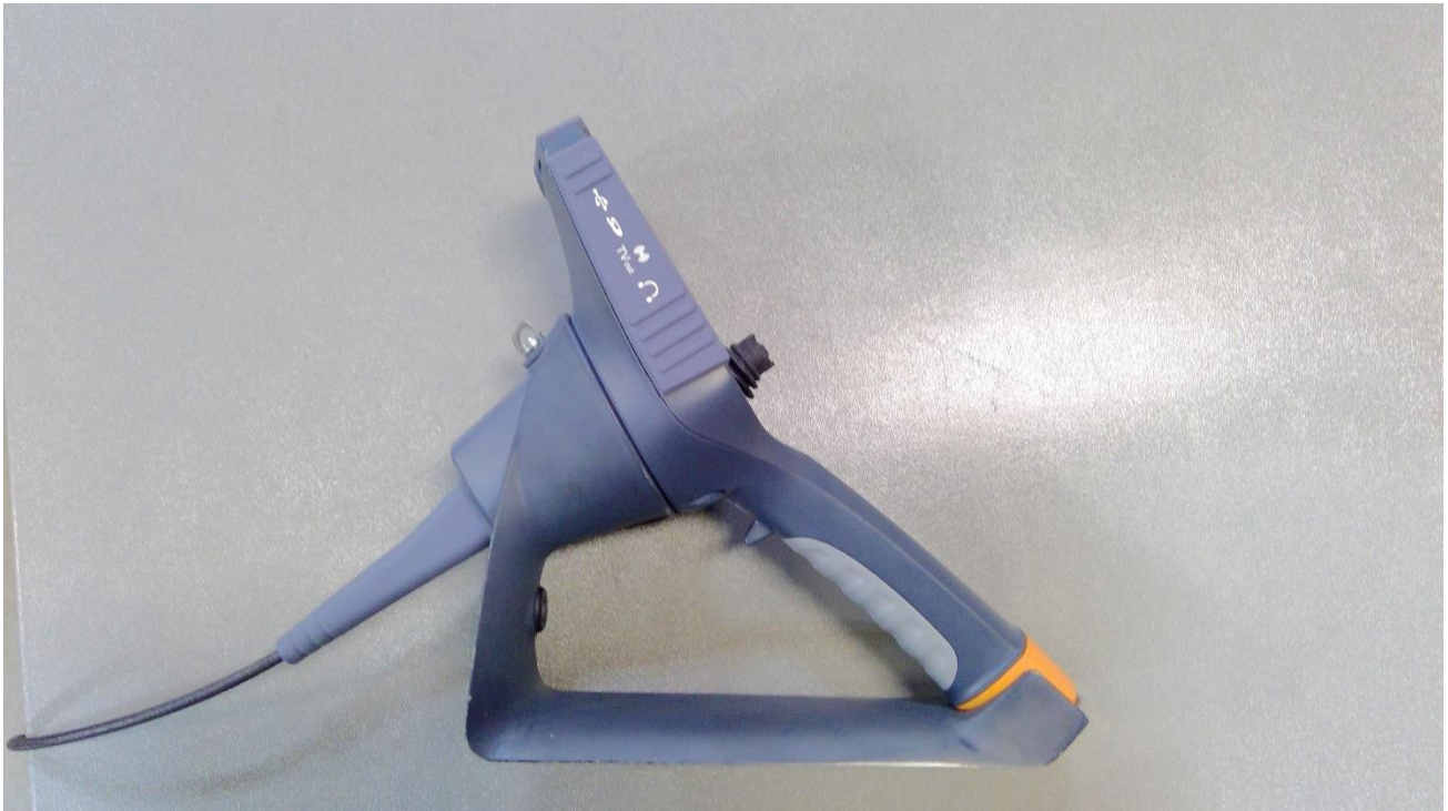
Figure 18: Test hardware after explosive atmosphere – Side 1
