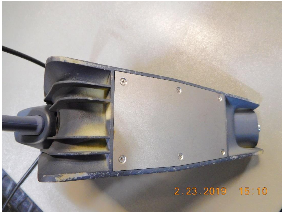
Figure 2: Test hardware before explosive atmosphere – bottom
