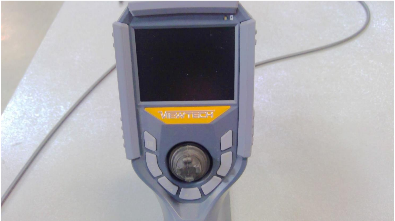
Figure 17: Test hardware after explosive atmosphere – screen, joystick
