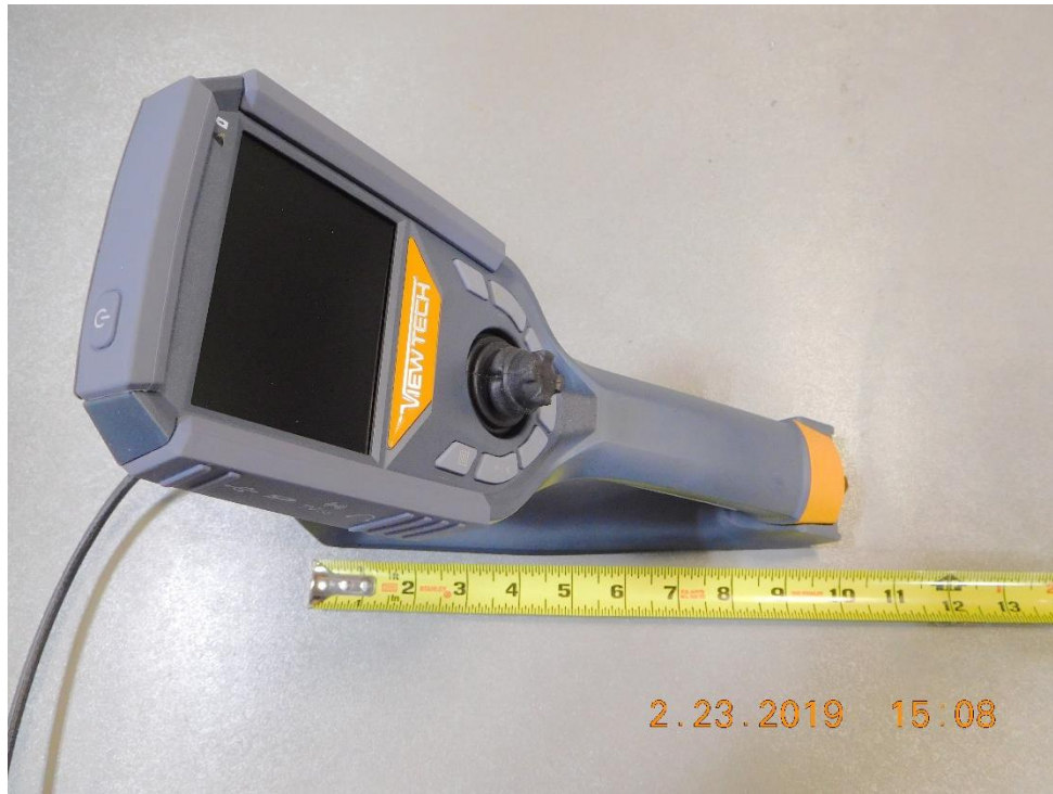
Figure 3: Test hardware before explosive atmosphere – handle, screen
