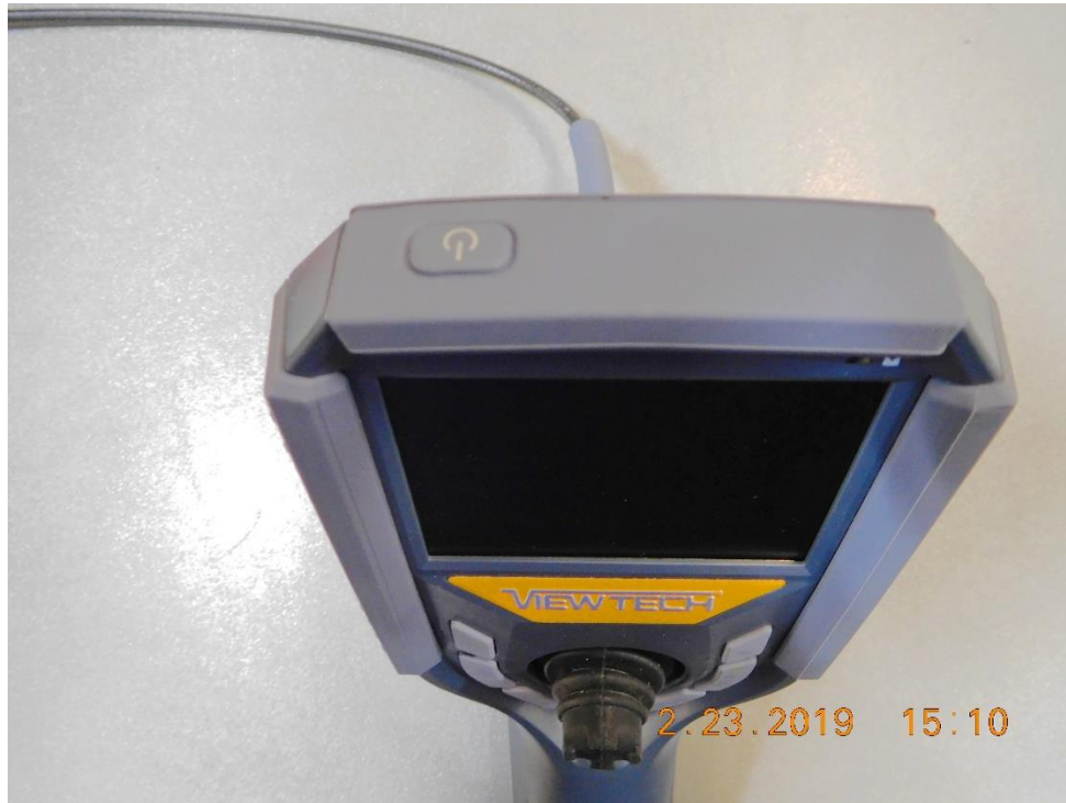
Figure 6: Test hardware before explosive atmosphere – power button, screen
