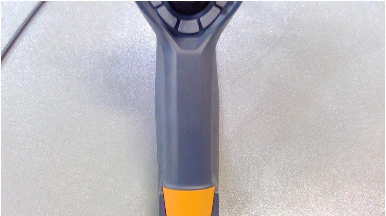
Figure 16: Test hardware after explosive atmosphere – handle
