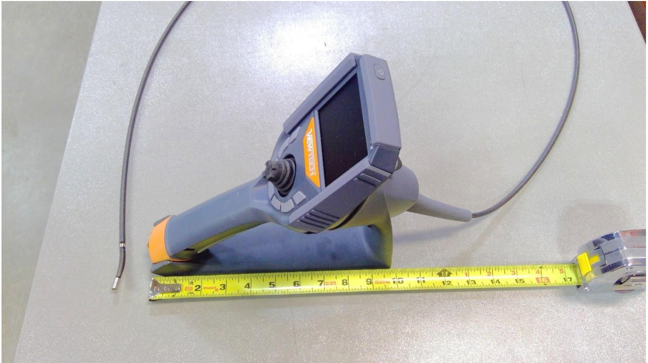
Figure 15: Test hardware after explosive atmosphere – handle, screen
