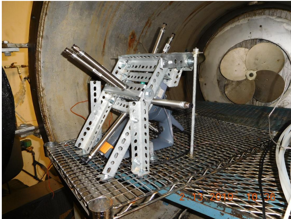
Figure 12: Explosive atmosphere test setup – test hardware installed in test chamber
